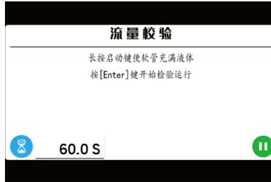
Make sure the tube is full of liquid, press and hold
