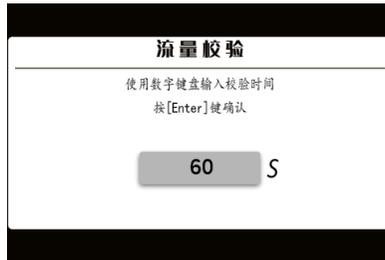
Use the numeric keypad to enter the calibration time. After entering, press
