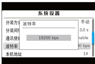
Press **▲** **▼** to select the baud rate, press **Enter** key to save and return to the system settings interface.
