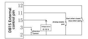
Description: The external control signal controls the direction, start and stop, and the analog signal controls the speed.
